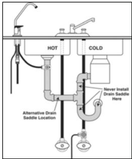
Figure 10: Drain Saddle Assembly Mounting Locations
